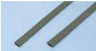
● Backup Material A polyethylene foam material placed in spaces between G Base and wall, frame for entrance/exit, etc. Specifications (in mm): 5.0mm (width) × 1,000 (length) × 20mm (height) Packing: 50 pieces/case
