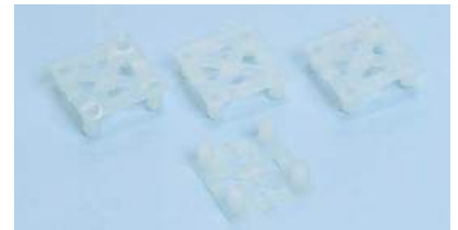
● X Joint Connects G Bases together. Useful for creating an accurate pitch between bases. Specifications (in mm): 26.4mm × 26.4mm × 8mm (height) Packing: 500 tiles/case (30m 2 )
